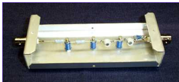
Inside the Attenuator
